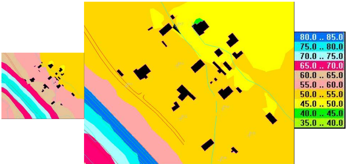
Figure 2: Nocturnal acoustic map without screens (left) and with screens (right) - Janodembra.
